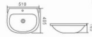
P20 Hang-Basin Size: 510×405×165mm Fixing with back to wall Vitreous china
