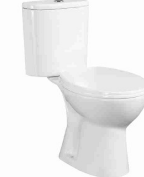
8315 Washdown Separated Toilet Bow & Tank Size: 645x365x770mm S-trap, 250mm Roughing-in P-trap, P-trap45°
