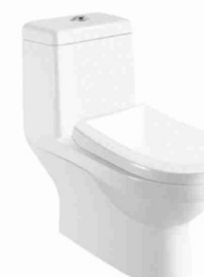
821 Siphonic One-piece Toilet Size: 510 x 290x490mm S-trap,190mm Roughing-in
