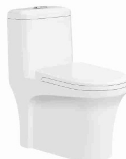
385 Siphonic One-piece Toilet Size: 680 x 360 x 745mm S-trap,300mm Roughing-in
