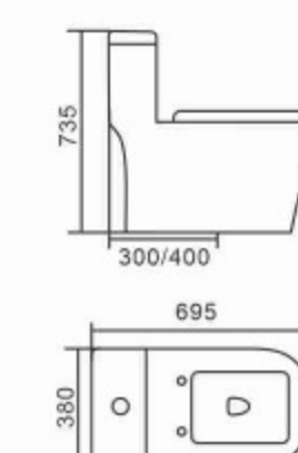
305 Siphonic One-piece Toilet Size: 695x380x735mm S-trap,300/400mm Roughing-in
