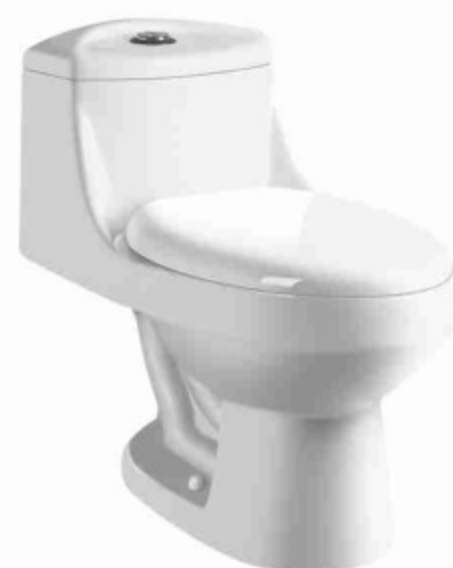
316 Siphonic One-piece Toilet Size: 710 x 385 x 640mm S-trap,300mm Roughing-in
