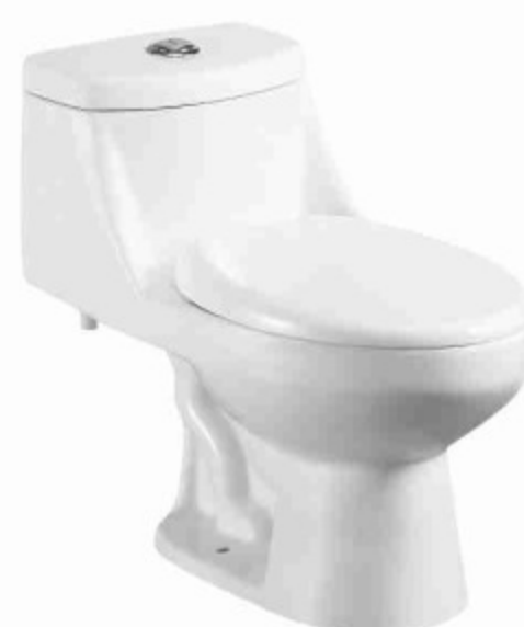
316B Siphonic One-piece Toilet Size: 710 x 385 x 640mm S-trap,300mm Roughing-in
