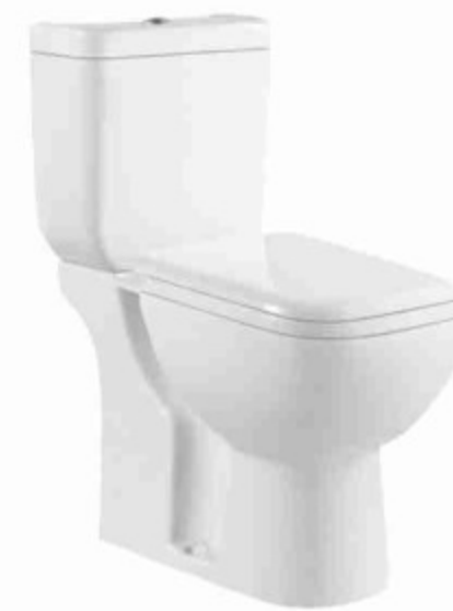
811 Washdown Separated Toilet Bowl & Tank Size: 645x350x800mm S-trap, 250mm Roughing-in P-trap, 180mm Roughing-in
