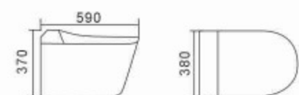
704 Washdown Wall hung closet Size:590x380x370mm Vitreous china
