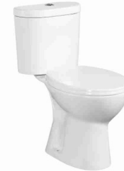
8318 Washdown Separated Toilet Bowl & Tank Size: 660x380x740mm S-trap, 250mm Roughing-in P-trap, P-trap45°
